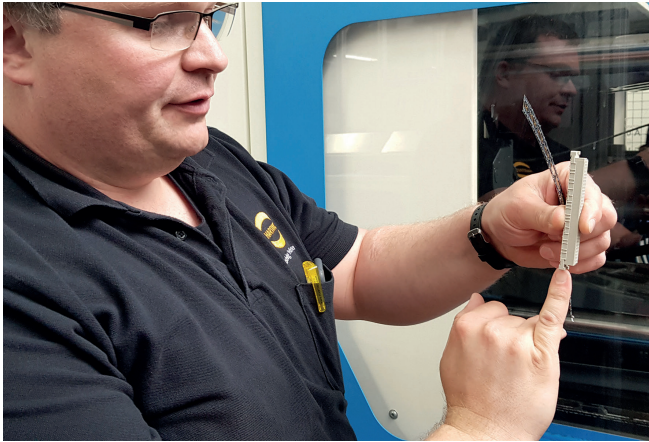
Fig. 3. "Lined up end to end, the 85 contact segments form the back-plane for the printed circuit board," explains Mark Gosewehr © Günther/ H. Wollstadt
